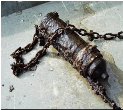
Sonic receiver used to monitor movement of fish implanted with sonic tags.
